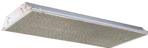
TA, FA series SMALL CELL louver: 1/2" x 1/2" x 1/2" cell specular silver parabolic louver, PL1. 44° shielding from all angles, excellent brightness control.
