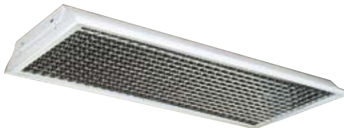
TS, FS series 1 1/2" supercube louver: 1 1/2" x 1 1/2" x 1" cell specular silver parabolic louver, PL2. 38° shielding from all angles, excellent brightness control.
